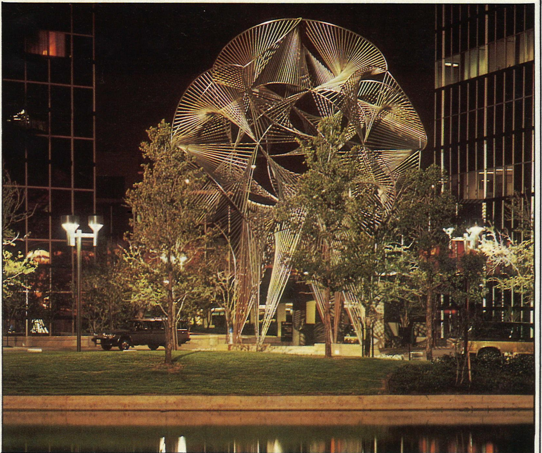
Only three compact source iodide fittings floodlight the Equinox sculpture in an office centre in Dallas, Texas; an example shown by Brian Page, Thorn Lighting, in his talk on discharge lamps.
